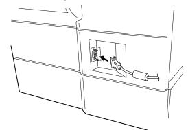
$\widehat{\mathcal{O}}$  Insert the female end of the PC interface cable into the serial (RS232C) port on your computer. Tighten the attached screws with a screw-driver.
