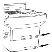
$\ensuremath{\overline{\mathcal{T}}}$  Rotate the received document tray back. Grasp the hand hold on the original document IN tray as shown, and open it.
