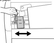
③ Push the pressure plate down until it locks into position.
