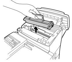
③ Pull the old drum cartridge out of the compartment.
